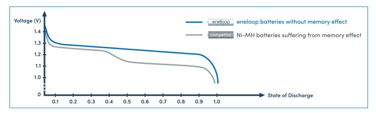
When a rechargeable battery that hasn't been fully discharged, is repeatedly topped up, it "remembers" that it's only been used for a short time. When used again, the voltage may quickly drop. This is called the memory effect. eneloop has a high voltage to begin with and so it maintains enough voltage even if this occurs. There's no need to worry about the memory effect.
